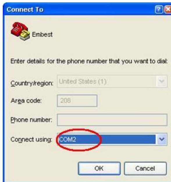
Figure 2-4 Select a COM port for connection
