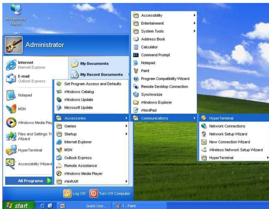
Figure 2-2 Create a new HyperTerminal
